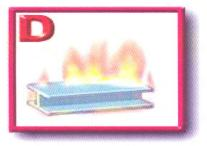
**Class D** - Extinguish combustible metals such as magnesium, titanium, potassium and sodium with dry powder extinguishing agents specially designated for the material involved.
